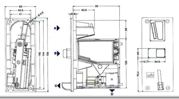
**Note:** All the dimensions are in millimeter.
